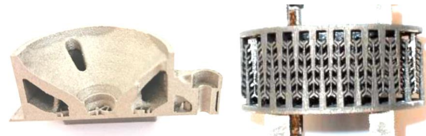
Base plate and flexible thermal structure made of ALSi10Mg, Mašek 2022
